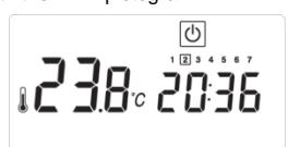
To activate the product, put the switch on « I » position. During 3 seconds, the software version will be displayed. Then, the thermostat comes back in the selected operating mode before the standby.
