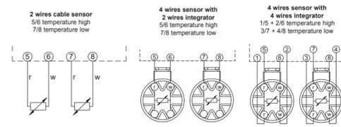
Wire cross section for head sensors ≥ 0,5 mm² (EN 1434-2)
