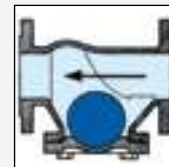
HORIZONTAL MOUNTING Lodging of the ball below the axis. The arrow shows the direction in which the liquid is rising.
