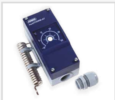
MVTH Room thermostat for powering self-regulating heating cable. In IP54 case. Measuring range -10 to 40 °C Differential 1-2 K. Power supply 230 Vac Contact 16A/230 Vac
